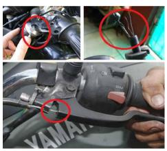
Figure 1. Damage on mechanical clutch
