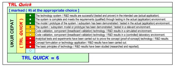
Figure 7. Quick TRL measurement by Techno-meter
