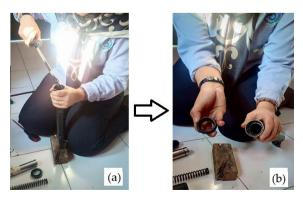
**Figure 5.** Photographic view of product testing by the author: the process of removing seal (a) and removed seal (b)
