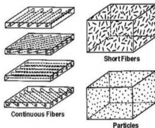
Figure 1. Illustration of composite material [10]
