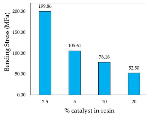
Figure 6. Bending stress to % catalyst in resin
