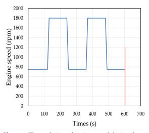
**Figure 3.** The evolution of engine speed during the test (The vertical red line in the 600th second indicates the cease of fuel pump operation)
