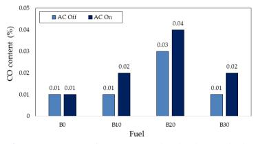
Figure 5. Comparison of CO emission with and without AC load.
