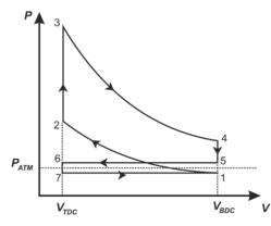
Figure 1. Indicated cycle and strokes
