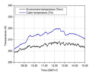
**Figure 6**. Profiles of the temperature inside the cabin and in the environment with a mini air cooler and exhaust fan
