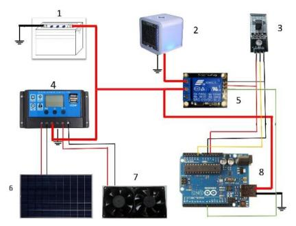
Figure 3. Cooling system circuit scheme (1. Battery, 2. Mini air cooler, 3. Temperature sensor, 4. Solar charge controller, 5. Relay, 6. Solar cell, 7. Exhaust fan, and 8. Micro-controller)
