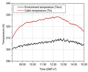
**Figure 5**. Profiles of the temperature inside the cabin and in the environment without a mini air cooler and exhaust fan
