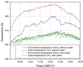
**Figure 7**. Profile of temperature difference inside the cabin with and without a mini air cooler and exhaust fan
