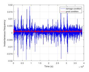
Figure 9. Instantaneous frequency extraction of damage and good condition vibration based on Hibert transform
