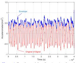
Figure 8. Envelope of the vibration signal on the alternator when operating at 750 rpm based on hibert transform
