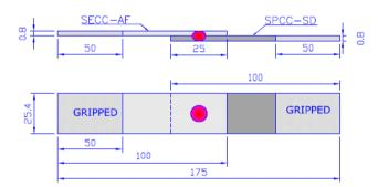
Figure 3. Tensile shear test geometry according to ASTM D1002
