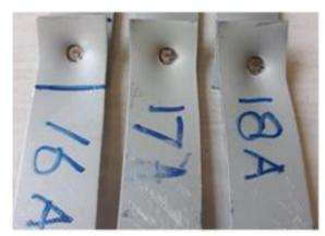
**Figure 8.** Pull-out failure mode for iteration 16, 17 and 18
