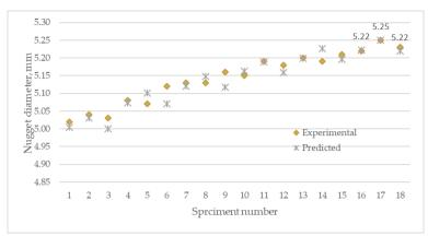
Figure 7. Predicted and experimental values of nugget diameter
