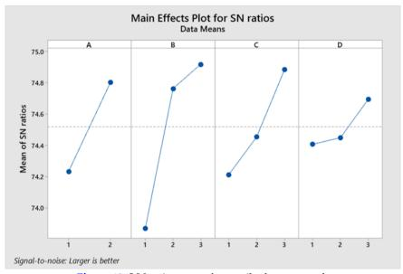
Figure 10. S/N ratio output for tensile shear strength
