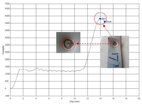
Figure 9. The highest tensile shear strength (force) result
