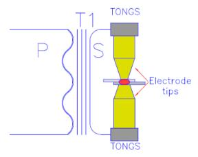
Figure 2. Schematic of resistance spot welding
