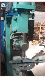
Figure 4. RSW machine 35 kW capacity
