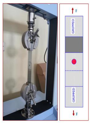
**Figure 5**. Tensile shear strength test of the coupon on UTM
